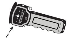
The sensitivity control trimpot is located directly infront of the Battery Recharger/ Earphone Jack
