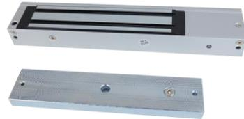
The DS-K4H255S Single-Door magnetic lock is designed for wooden door, glass door, and metal door. Aluminum is the main material. The maximum thrust of the lock is 272 kg (600 Lbs). It can be used for controlling door opening/closing. Special anti-residual magnetism designed makes the access control automation safer and electric lock more durable.
